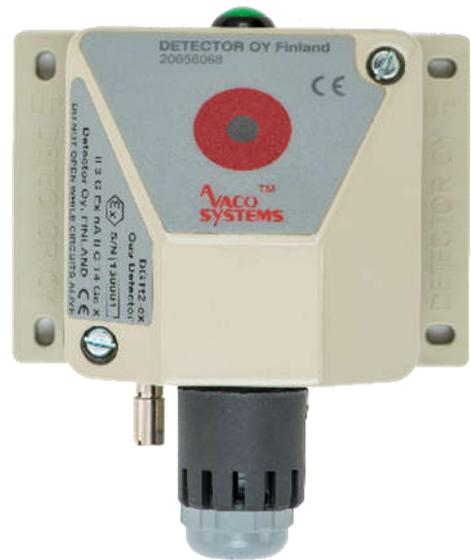
Enclosure dimensions: 89 mm x 89 mm x 69 mm. The enclosure base can be turned up side down for the wires. Installation depending of the controlled gas. Enclosures, DGT-t2w (in the picture) for wall-, DGT-t2d for duct and DGT-t2c for ceiling installation. Easy mounting due to the isolating/mounting plate.
